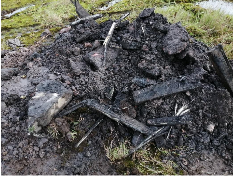
Photograph 13.1 Black staining on the soil in TP04. Significant anthropogenic waste in the pit, such as timber and concrete blocks.
