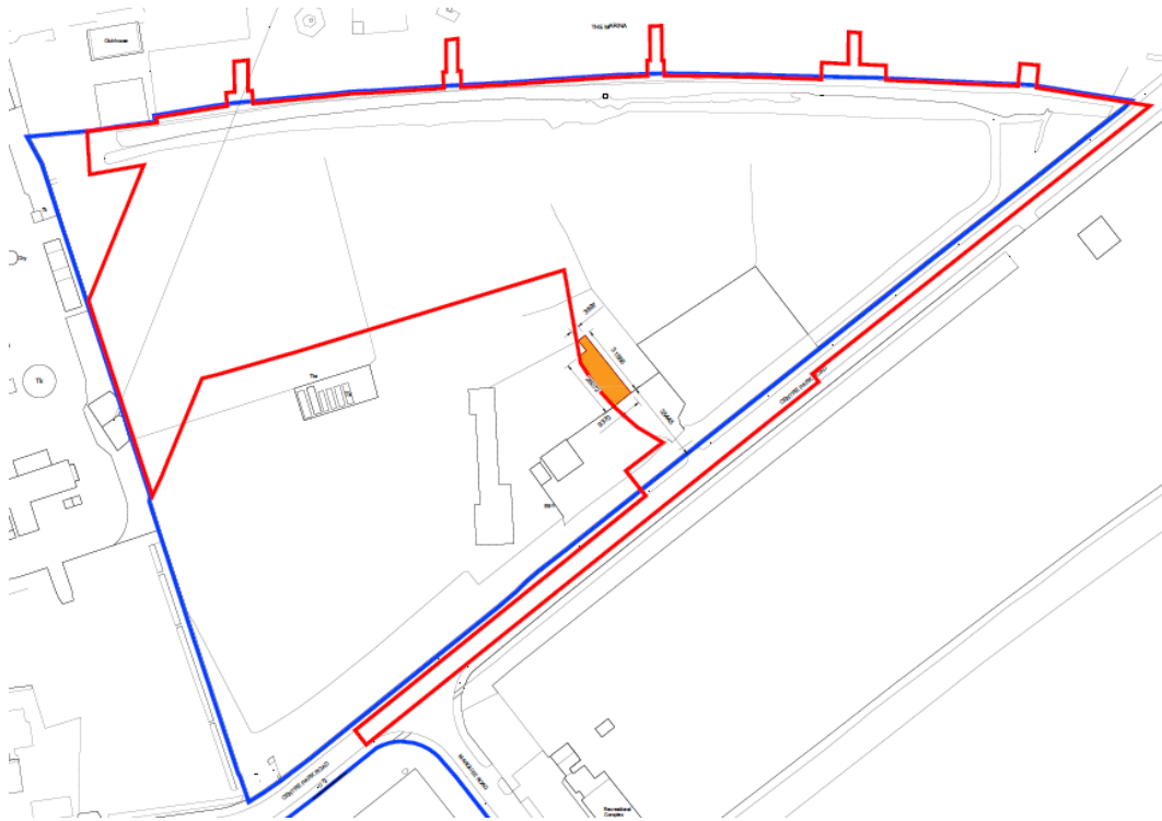
Figure 15.4: Existing Buildings and Structures – Extract from Demolition Plan – North Site, Drawing No. PE21055-CWO-ZZ-00-DR-A-0101 | not to scale
